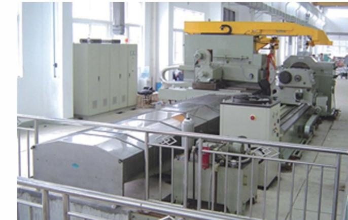
Workpiece and grinding wheel machine beds use vibration isolation design for large-sized machine bed, namely workpiece and grinding wheel machine beds are separated, which can avoid the mutual effect between the independent shaking resources of the workpiece machine body and grinding wheel machine body.
